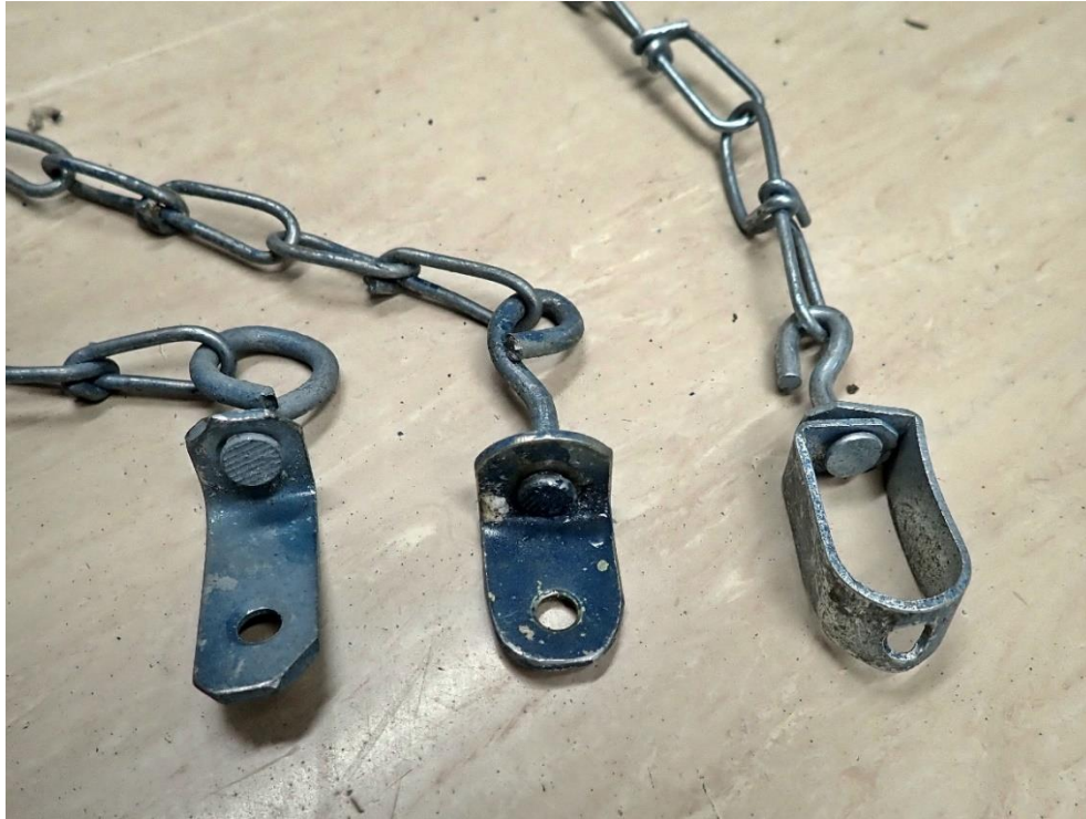
Figure 2. The swivel on the end of the chain of the 2-spring, 1-spring, and 0-spring traps, respectively.
