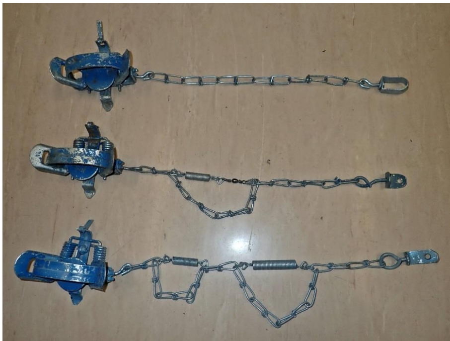
Figure 1. The three trap types used in this study; from top to bottom: standard No. 1 trap (0-spring), 1-spring modification, and 2-spring modification.
